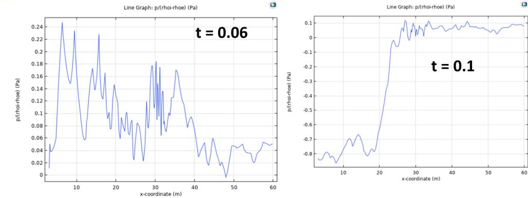
Fig. 3. Comparison of density wave oscillation inside the tube and reservoir (crack) at different time instances. Plane decompression wavefront moves in the opposite direction as the wave exits the conduit, it reflects after hitting the sound hard (No flow) wall. The wave front is rarefracted back as it approaches the exit due to higher impedance difference in the reservoir with  $m = 10^{-10} \text{ kgs}^{-1}$
