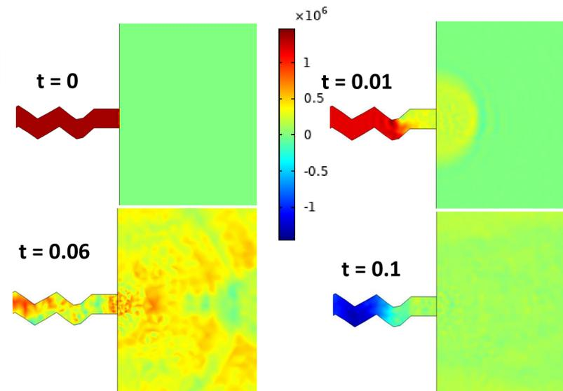
Fig. 2. Surface plot of the different acoustic wave regimes when the rocks are cracked. Large conduit to crack ratio (14)
