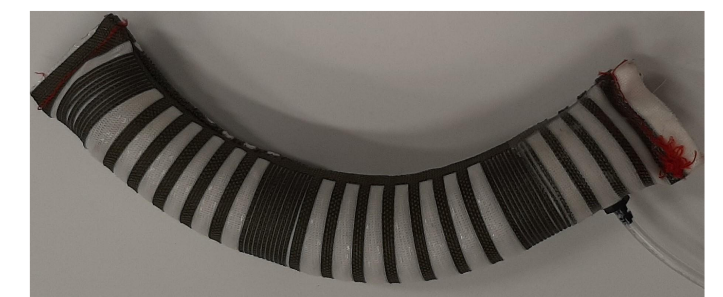
Pneumatic actuator when P=20psi
