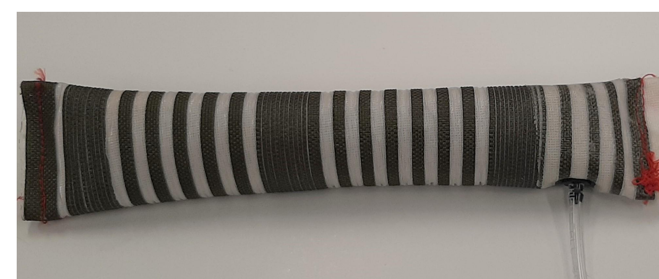
Pneumatic Actuator in ideal state(P=atm)
