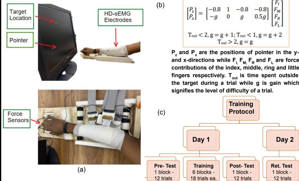
Figure 2: (a) Experiment Setup (b) Equations Used to Develop Training Protocol (c) Experiment Design
