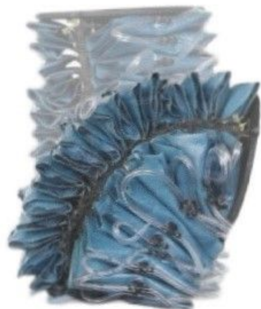
Fig 1: Soft Arm Manipulator Bending: Changing the pressure in the robots' three pressure chambers allows the robot to bend.
