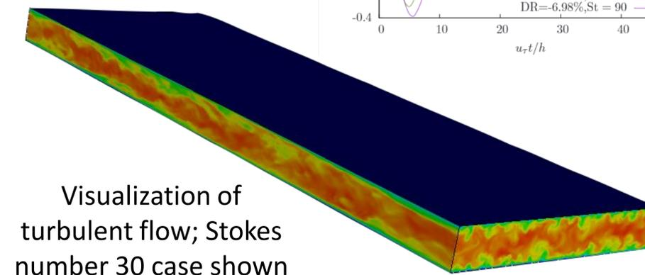
Visualization of turbulent flow; Stokes number 30 case shown
