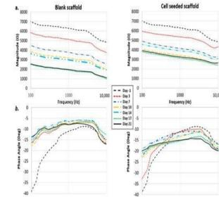
Impedance magnitude and phase over current frequency with and without cells and compared with different growth times<sup>4</sup>.
