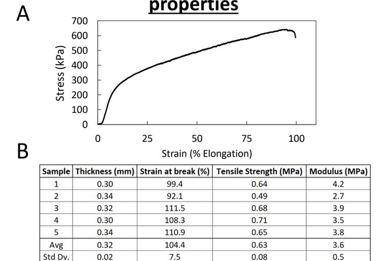
**Figure 4:** (A) Stress-strain curve for a scaffold spun at 10% mandrel speed. (B) Five samples at 10% speed were tested. Average Young's modulus was found to be  $3.6 \pm 0.5$  MPa, the tensile strength was found to be  $0.63 \pm 0.08$  MPa, and the strain at break was found to be 104.4% of the original length.
