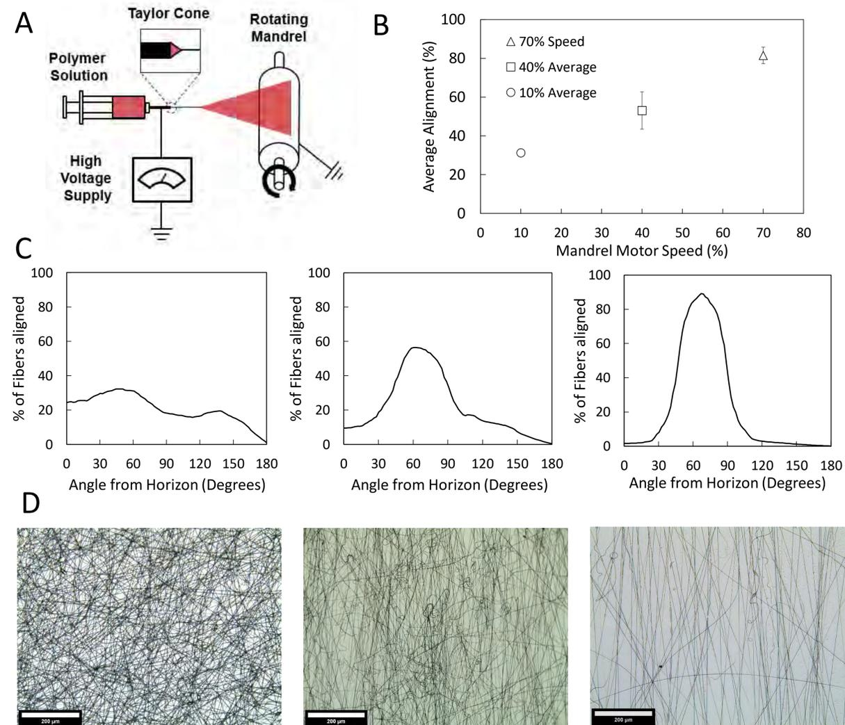
**Figure 3:** Alignment of electrospun fibers can be controlled by electrospinning onto a rotating collector. (A) Electrospinning apparatus with rotating drum. (B) Fiber alignment as a function of mandrel velocity confirming fibers are more aligned as mandrel speed increases. (C) Distribution of fiber alignments for 10, 40, and 70% motor speed (left to right). (D) Brightfield images (scale 200µm) of scaffolds for 10, 40, and 70% motor speed (left to right).
