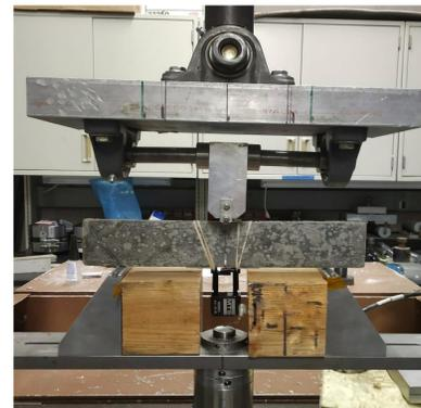
3 point bend test set up
