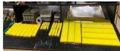
Plexiglass molds used for cement beam castings
