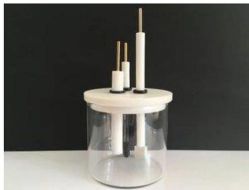
Figure 1 | three-electrode experiments
