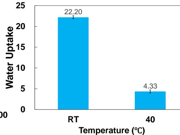
Fig. 5 The water uptake of optimized PNIPAAm hydrogel at 40 °C.
