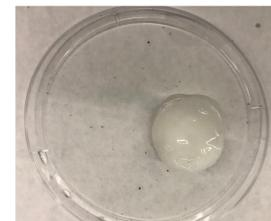
Fig. 7 Optimized PNIPAAm hydrogel at RT
