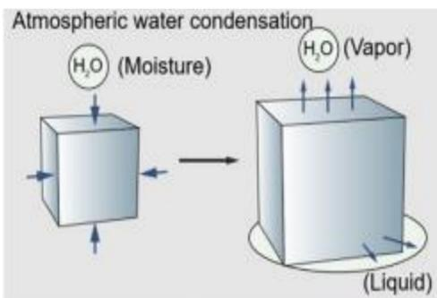
Fig. 1 The atmospheric water capturing and releasing processes via moisture absorbent [1]. The process of moisture from the air will be release in liquid form through the condensation. The hydrophilic polymer-based hydrogel network works as a platform to store gaseous water.
