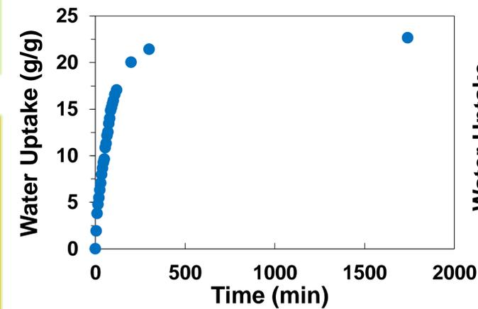
Fig. 4 The water uptake of optimized PNIPAAm hydrogel at room temperature.
