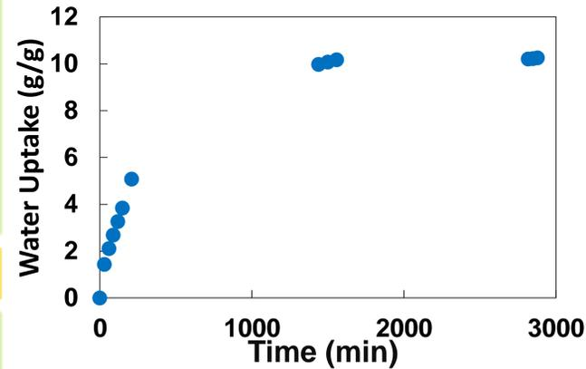
Fig. 2 The water uptake of PNIPAAm hydrogel at room temperature
