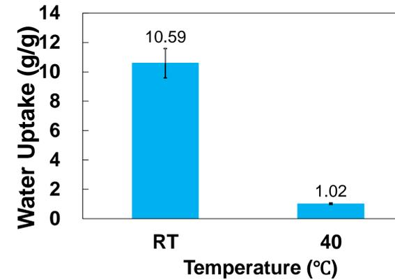
Fig. 3 The water uptake of PNIPAAm hydrogel at 40 °C.
