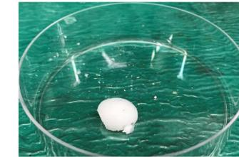
Fig. 6 PNIPAAm hydrogel at RT.
