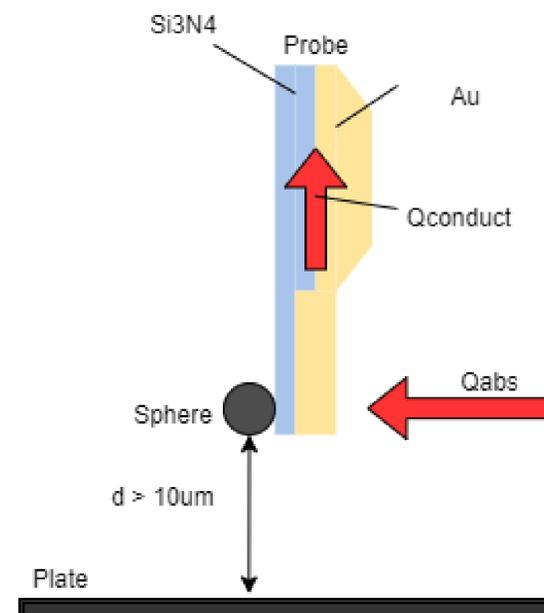
Figure 1: Heat Transfer Model of Probe and Plate out of effective range of NFR
