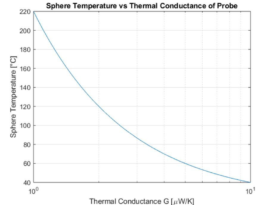
Figure 3: Theoretical Plot of Sphere Temp vs Thermal Conductance of AFM Probe; No NFR Heat Transfer
