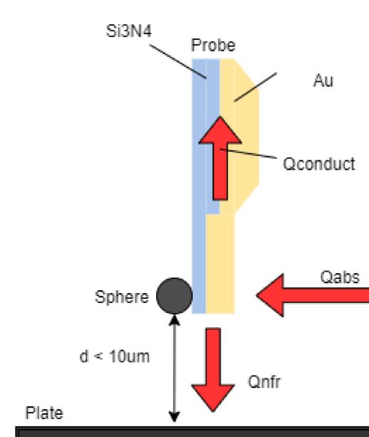
Figure 2: Heat Transfer Model of Probe and Plate within range of NFR
